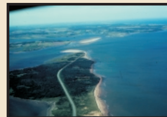
Rustico Bay and Rustico Inlet illustrating erosional termination of Coastal Highway and landward movement of the entire barrier
