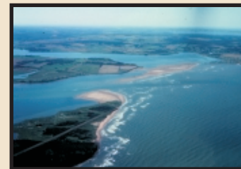
Rustico Bay and Rustico Inlet illustrating erosional termination of Coastal Highway and landward movement of the entire barrier
